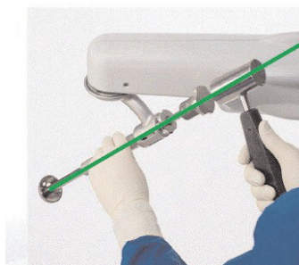
Figure 34. Robotic Arm Constraint during Cup Impaction
