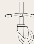
castors Ø 125 mm with central brake and directional castor (\*)
